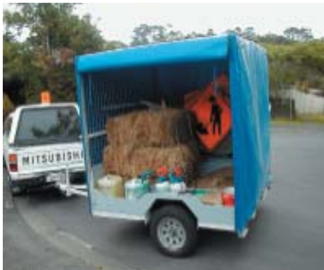
Figure 15: Wastewater overflow containment unit
