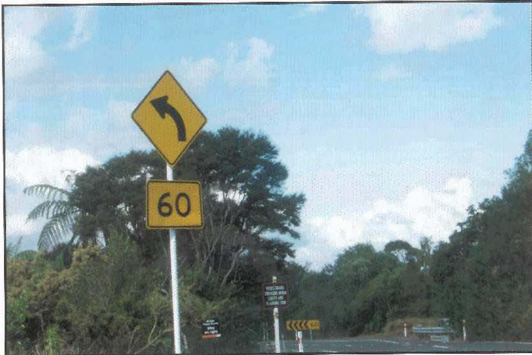
Photograph G: Advanced curve warning and horizontal curve chevron with non-standard advisory speeds of 60 kph.
