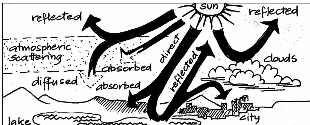
Solar energy is highest when the sun is overhead midday and summer. It is lowest when the sun angle is low e.g. sunset, or in winter, when it rises no more than 30 degrees above the horizon and the radiation has to pass through the atmosphere for a much greater distance.
