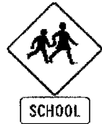
Standard school warning sign
